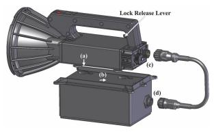
**Lock Release Lever** under the searchlight handle, then slide searchlight forward away from battery connector end.
